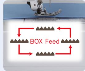
The BOX Feed system stays in contact with your fabrics longer for a consistent, reliable seam every time.
