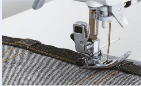
**Thick denim folded into three layers for a flat fell seam**
