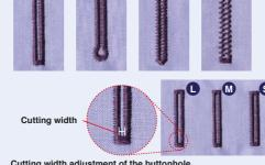
Cutting width adjustment of the buttonhole Now it is possible to adjust the cutting width in 3 steps
